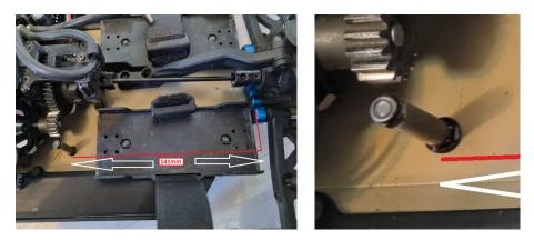
Remove the Speedo tray from the buggy and then cut away the area on the radio box as per the photos. Do this until you have enough clearance for the speedo to sit in front of the battery stop screw. Depending on what Receiver you use will dictate if you can still fit the top half of the radio box.
